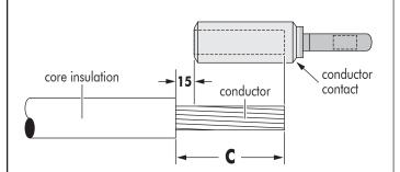
A. Remove the core insulation from the conductor for a distance **« C »** mm
