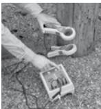
Fluke-1625 Earth Resistance Testing
