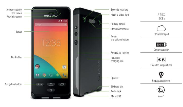
The BARTEC PIXAVI Impact X is the toughest smartphone you will ever meet. This intrinsically safe smartphone has all the functionality you will expect from a regular smartphone. The ATEX and IECEx certification has not compromised the quality and usability. The device is explosion proof and rated for use in hazardous areas. The Impact X is the next generation wireless video communication technology from BARTEC PIXAVI.
