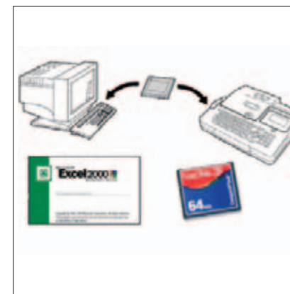
WITH THE HELP OF EXCEL AND A COMPACT FLASH CARD YOU CAN TRANSFER DATA FILES FROM YOUR PC TO THE PROMARK.
