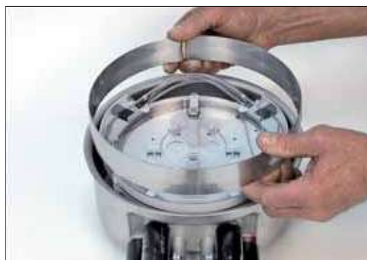
Mounting of support sleeve
