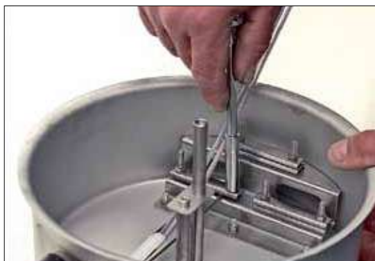
... and closing of strain relief clamp
