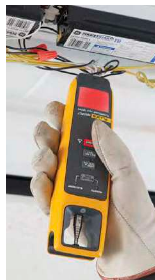
Non-contact voltage: Quickly check for voltage presence
