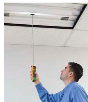
Lamp test: Test bulb without removing from fixture
