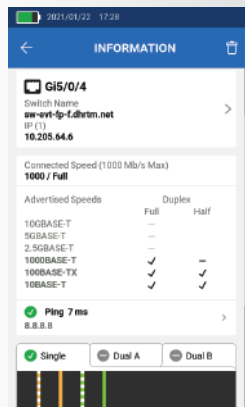
Switch port test shows switch name and IP address, connected port, and VLAN along with advertised speed and duplex settings. If a ping test is configured, the target address and average response time are shown. Scrolling down displays Power over Ethernet results.
